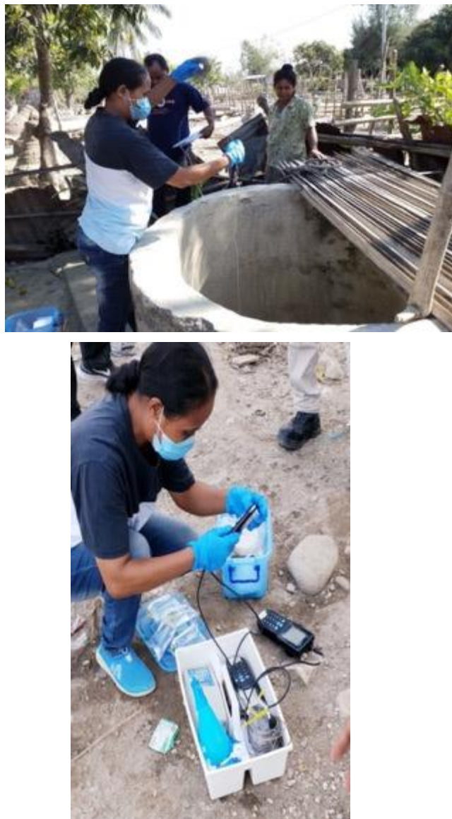
Figure 6-34. Example of Ground Water Sampling and Onsite Tests with HACH Instruments
