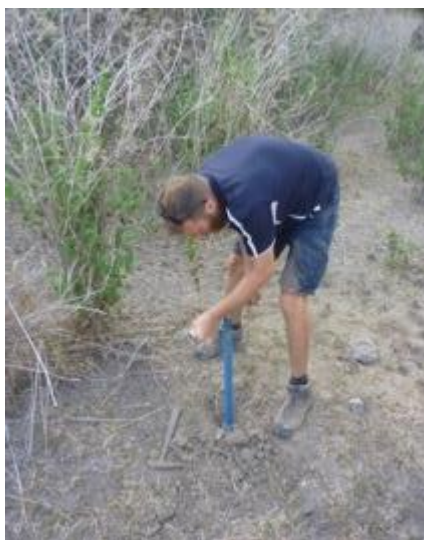
Figure 6-38. Field soil sampling using Auger hand drilling
